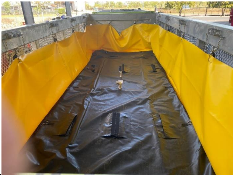
Figure 6: 10,000 litre IBC Bladder prior to filling
